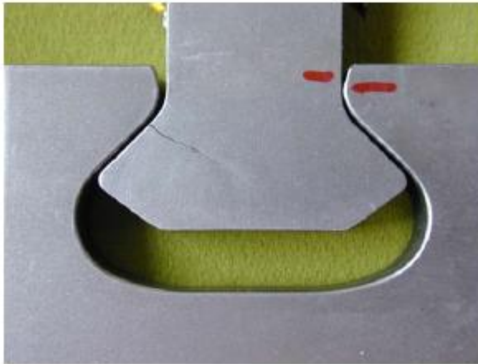
FIGURE 3. Failed specimen from biaxial dovetail rig.
