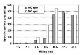
5 Specific surface area in milled coke powders after milling at 400 and 600 rev min<sup>-1</sup> for different times
