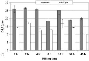
3 Evolution of a D50 and b D4·3 parameters in milled coke powders after milling at 400 and 600 rev min<sup>-1</sup> for different times
