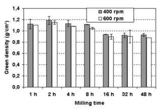
8 Green density in milled coke powders after milling at 400 and 600 rev min<sup>-1</sup> for different times, and CIP processing
