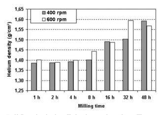
7 Helium density in milled coke powders after milling at 400 and 600 rev min<sup>-1</sup> for different times
