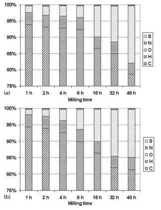
10 Chemical analysis of milled coke powders after milling at a 400 and b 600 rev min<sup>-1</sup> for different times
