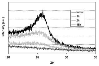
2 X-ray diffractograms of milled coke at 400 rev min<sup>-1</sup> for different times
