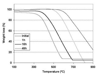
9 Thermogram in air of milled coke powders after milling at 400 rev min<sup>-1</sup> for different times
