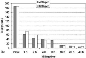
11 Atomic a C/H and b C/O ratios in milled coke powders after milling at 400 and 600 rev min<sup>-1</sup> for different times
