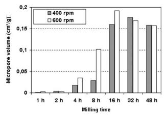
6 Volume of micropores in milled coke powders after milling at 400 and 600 rev min<sup>-1</sup> for different times
