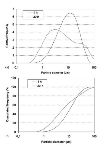
4 Sieve analysis of milled coke powders during 1 and 32 h at 600 rev min<sup>-1</sup>: a relative and b cumulated frequencies
