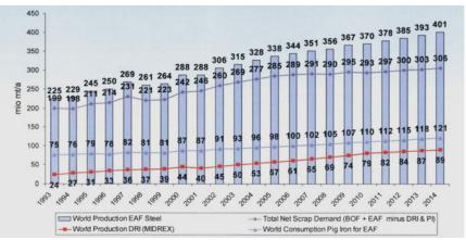
Fig. 3 Pig iron and DRI for EAF steel production (source: IISI and SGL Group internal figures)
