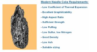
Fig. 15 Key quality properties for needle coke
