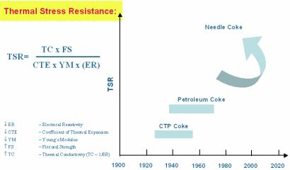
Fig. 9 Steps in raw material based graphite electrode quality expressed by thermal stress resistance
