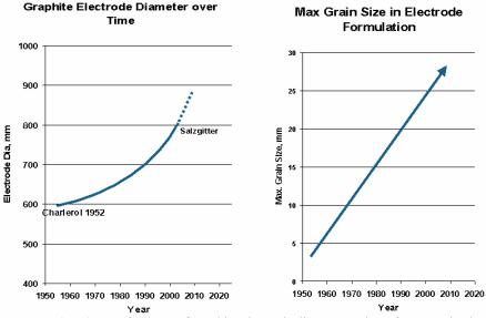
Fig. 12 Development of graphite electrode diameter and maximum grain size
