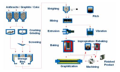
Fig. 10 Manufacturing of graphite electrodes
