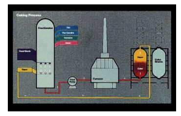
Fig. 10 Delayed coking process
