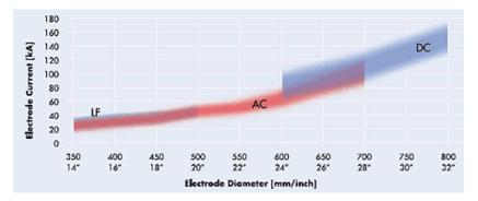
Fig. 5 Electrode current and required electrode diameter
