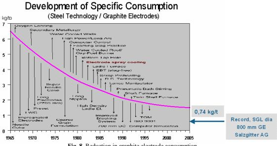
Fig. 8 Reduction in graphite electrode consumption
